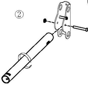
Rotate the tube to select eyelet facing upwards.
