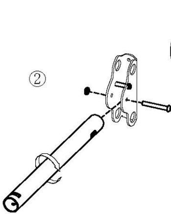
Rotate the tube to select eyelet facing upwards.
