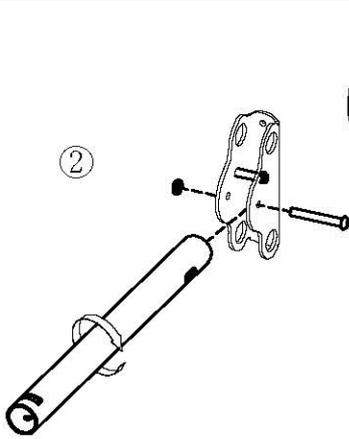
Rotate the tube to select eyelet facing upwards.
