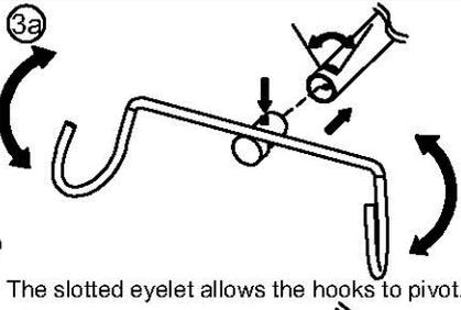
The slotted eyelet allows the hooks to pivot.
